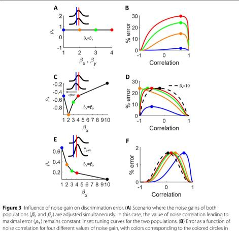
noise correlation for four different values of noise gain, with colors corresponding to the colored circles in panel "A". Filled circles indicate  $\rho_*$ . (**C**) Impact of modifying the noise gain of population x only. (**D**) Different values of noise gain for population x. (**E**) Scenario taken from panel D of Fig. 2, showing a monotonic decrease in  $\rho_*$  when increasing  $\beta_x$ . (**F**) Impact of  $\beta_x$  on classification error
